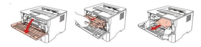
**Step3:** After taking out papers jammed, install the laser toner cartridge again and close the front cover, then the printer will recover printing.
